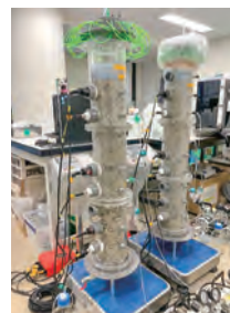
Leaching tests for excavated soils and rocks
